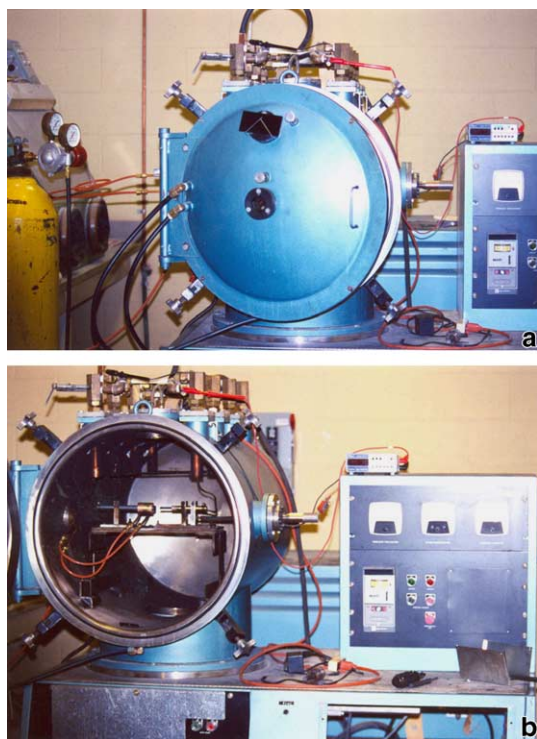
Fig. 1. Converted vacuum/pressure chamber for electric arc-discharge system. (a) Chamber exterior view. (b) Open chamber showing arc-discharge arrangement. The arrow shows the adjustable anode system.
