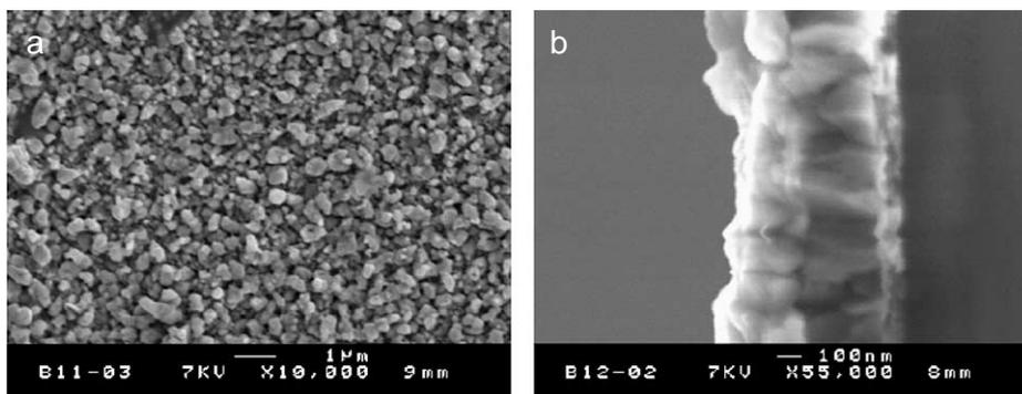
Fig. 2. (a) SEM and (b) cross-section of FeS<sub>2</sub> films sulphurated from iron oxide layers at 450 °C for 6 h under a vacuum of about 10<sup>-4</sup> Pa.
