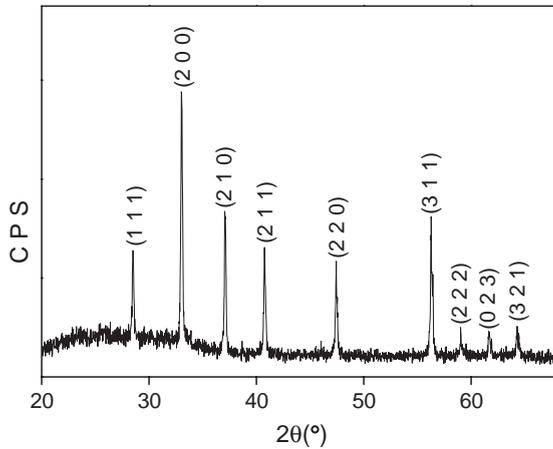
Fig. 1. XRD patterns of FeS<sub>2</sub>-pyrite thin films prepared under a vacuum of 10<sup>-4</sup> Pa for 6 h at 450 °C.
