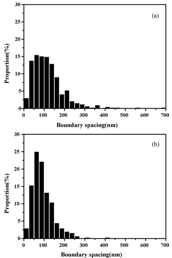
Fig. 2. The frequency histogram of lamellar boundary spacings of commercially pure Ni rolled at: (a) room temperature and (b) liquid nitrogen temperature, to a thickness reduction of 95%.
