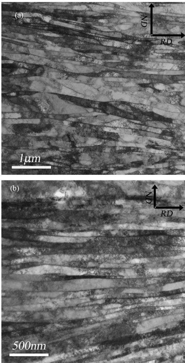
Fig. 1. TEM micrographs showing the deformed microstructure of commercially pure Ni after rolling at: (a) room temperature and (b) liquid nitrogen temperature to a thickness reduction of 95%.
