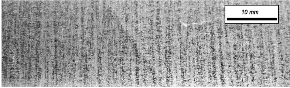
Fig. 1. Development of roping in an AA6111 sheet after a stretch of 15% elongation in the TD. The sample has been given “stoning treatment”, a light sanding of the surface by a piece of carborundum with silicone dry film lubricant, to enhance the visibility of the roped surface. The RD is vertical and TD is horizontal.
