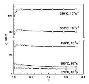
Fig. 1. True stress-true strain curves for the 5083 Al.
