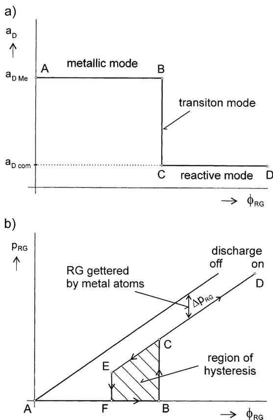
Fig. 1. Schematic illustration of (a) deposition rate,  $a_D$ , of sputtered films, and (b) partial pressure of RG,  $p_{RG}$ , as a function of flow rate of RG,  $\phi_{RG}$ .
