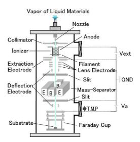
Fig. 1. Schematic illustration of the polyatomic ion beam system.
