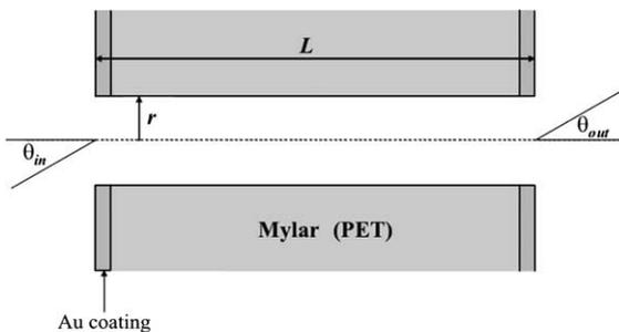
Fig. 1. Geometry of nanocapillary of length  $L$  and radius  $r$ . Ions enter at an angle  $\theta_{\text{in}}$  and exit at an angle  $\theta_{\text{out}}$  relative to the capillary axis.
