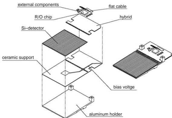
Fig. 1. Endcap preshower detector module.
