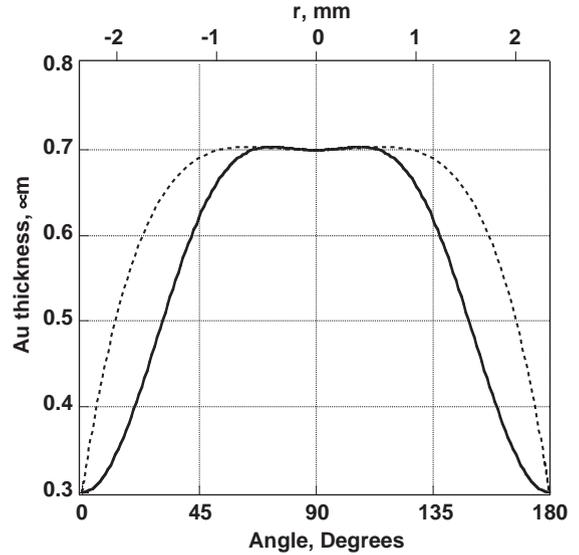
Fig. 1. Calculated shim profile (solid line—bottom axis) to zero out the P2 + P4 asymmetry of the SNL-Z double-ended pinch hohlraum drive. The projection (dashed line—top axis) of this profile on a plane containing the poles is also shown for future reference.
