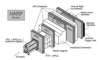
Figure 1. Schematic layout of the HARP spectrometer.
