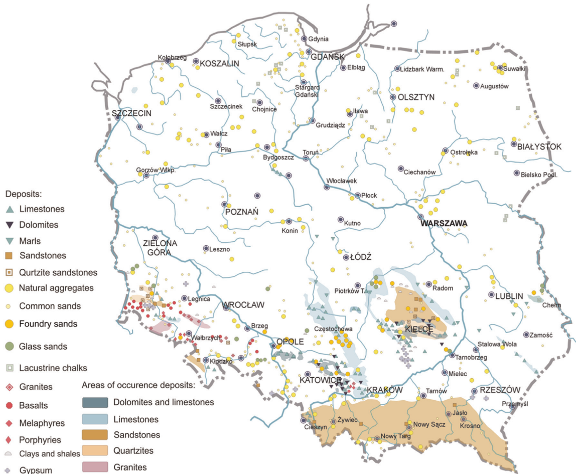
Fig. 1. Distribution of industrial rock deposits in Poland (generalized acc. E. Pietrzyk-Sokulska et al., in print);
