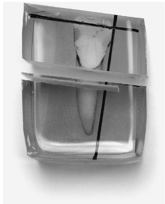
Fig. 3. Two cuts have been made perpendicular to the drawn line running parallel along the exterior of the root. The line perpendicular to that line is used as a guide for sawing. Later, for orientation during microscopy, the outer edge of the plastic slice where both cuts had hit the root perpendicular will be marked with a permanent marker.
