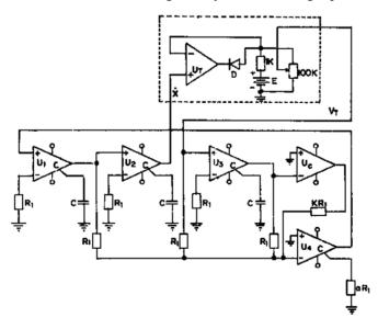
Fig. 1. Circuit implementation of Eq. (1), with the precision clipping control circuit depicted in the dotted box.  $V_T$  is the threshold controlled signal.
