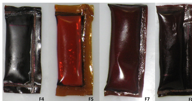
Fig. 1. Sealed samples packing palm oil for in-vivo shelf life evaluation (F4: maximum coffee and cocoa, F5: no cocoa, F7: no coffee and F8: maximum coffee).
