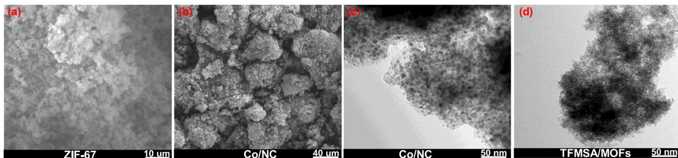
Fig. 1. Typical scanning electron microscopic images of (a) ZIF-67 and (b) Co/NC, and transmission electron microscopic images of (c) Co/NC and (d) TFMSA/MOFs.
