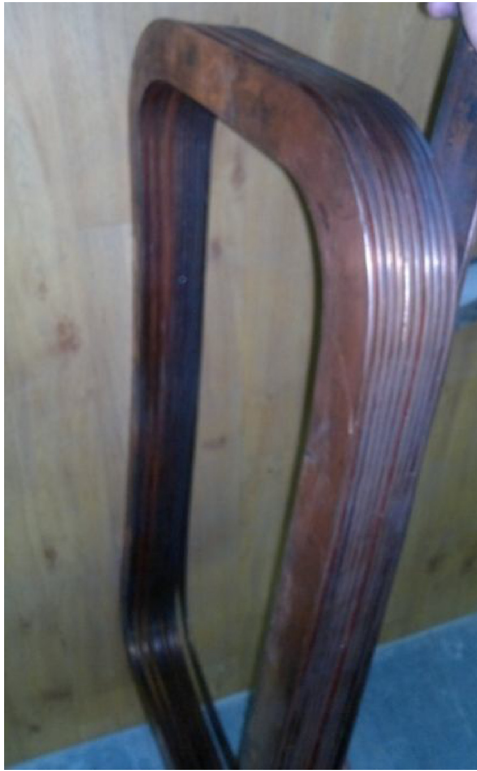
Fig. 1. A set of toroidal coils consisted of 10-loop belts in Alborz Tokamak.
