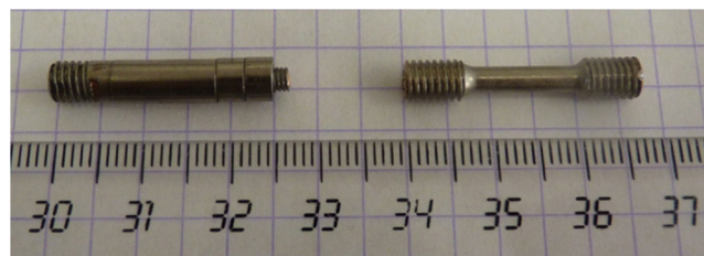
Fig. 1. Uni-axial pre-stressed and locked creep relaxation (left) and thermal creep test (right) Ni-coated specimens before irradiation.
