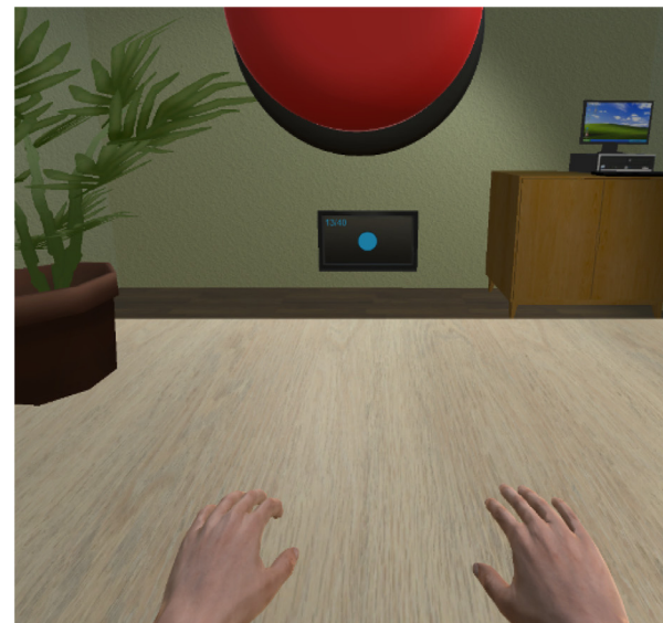
Fig. 1. Comparison of MI-BCI training environments. Left top – example of the Graz training paradigm with symbolic instructions (indicating the user should perform right hand MI), left bottom – feedback in Graz training (indicating detected right hand MI). Right – our embodied VR training environment. Participants try to move the virtual hands by using MI of left and right hand.
