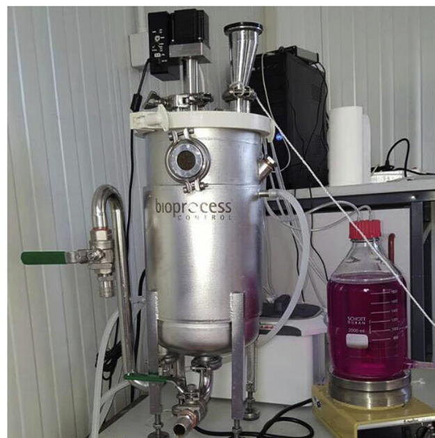
Fig. 1. Semi-pilot stainless steel reactor used for semi-continuous trials.
