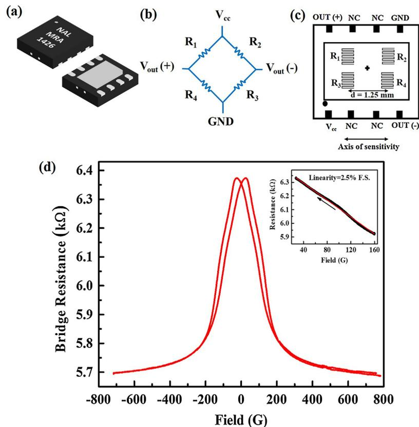
Fig. 2. (a) 8 T DFN packaged GMR gradiometer sensor, (b) Wheatstone bridge equivalent circuit of the GMR sensor, (c) configuration of GMR sensing resistors with respect to sensor package, and (d) measured GMR characteristics of a single resistor. The linear region extends from 40 G to 160 G (inset).
