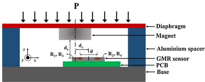
Fig. 1. Illustration of magnetic pressure sensing mechanism.
