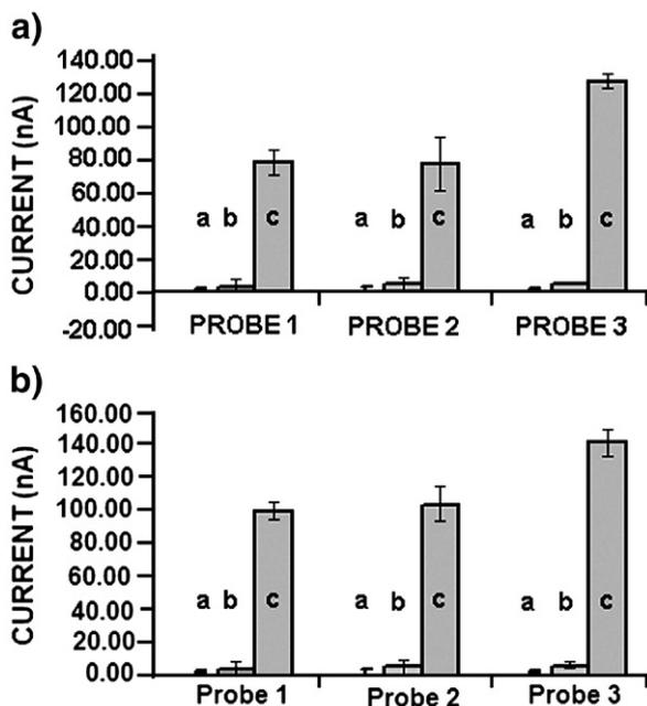
Fig. 4. Histammograms obtained from differential pulse voltammograms of guanine oxidation signals after probe immobilization by; a) electrostatically, b) covalently; a) before hybridization, after hybridization with; b) Non complementary PCR products (HSV real samples), c) HBV positive PCR products.
