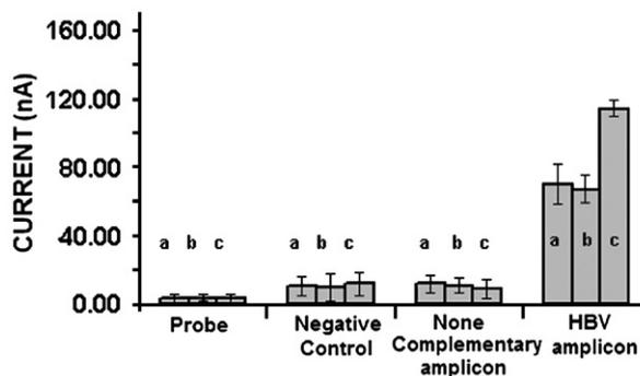
Fig. 5. Histammograms obtained from differential pulse voltammograms of guanine oxidation signals; a) Probe 1, b) Probe 2, c) Probe 3 modified PGE surfaces, before and after hybridization with positive HBV real samples, negative control samples, non complementary amplicon (HSV PCR products).
