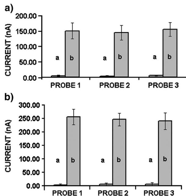
Fig. 3. Histograms obtained from differential pulse voltammograms of guanine oxidation signals after probe immobilization by; a) electrostatically, b) covalently attachment; a) before hybridization, b) after hybridization with complementary targets.
