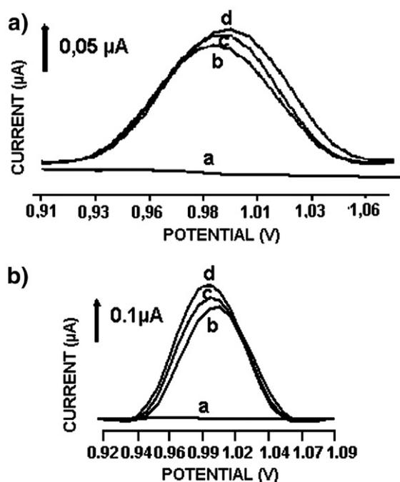
Fig. 2. Differential pulse voltammograms of guanine oxidation signals in acetate buffer solution obtained after probe immobilization by; a) electrochemically, b) covalently attachment; a) before hybridization, after hybridization between; b) hybrid (2Probe 2 with Target 2), c) hybrid 1 (Probe 1 and Target 1), d) hybrid 3 (Probe 3 and Target 3).
