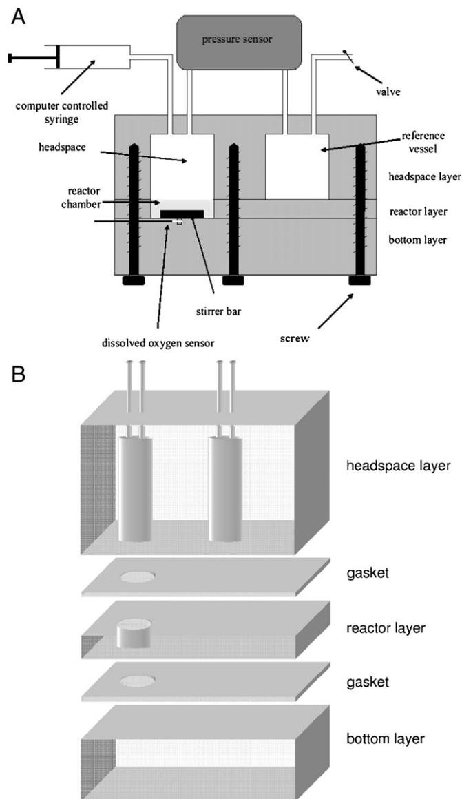
Fig. 1. (A) Schematic representation of the 100  $\mu\text{L}$  bioreactor, equipped with pressure based gas measurement system and (B) exploded view of the reactor.
