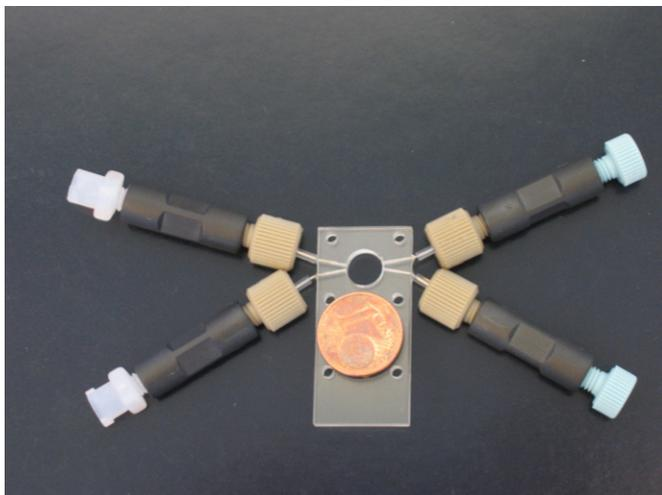
Fig. 2. Picture of the reaction chamber of the 100 µL bioreactor with fluidic connections.
