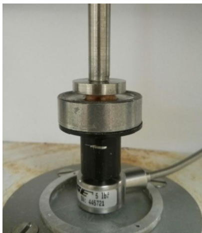
Figure 2 – Compressive DMA set-up for human bladder tumours.
