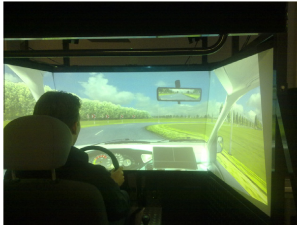
Fig. 1. The driving simulator that was used in the experiment. The dashboard shows the speed and engine rpm. Gear changing was automatic.
